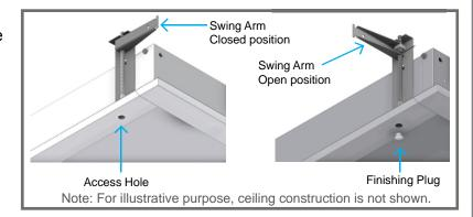
5). Seal all holes, gaps and entire perimeter of flange to plenum, caulk/sealant by others.
